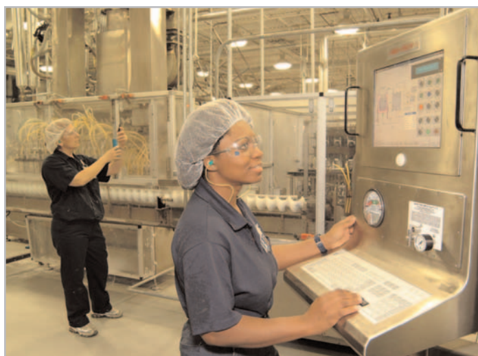
Empowering employees with the right level of technical skills and access to valuable job aids or tools necessary to effectively operate and maintain equipment is an important component of a strategic maintenance program. Operators at Unilever's Raeford, North Carolina, facility use Rockwell Software RSVIEW human-machine interface software to monitor the batch operation in real-time.
