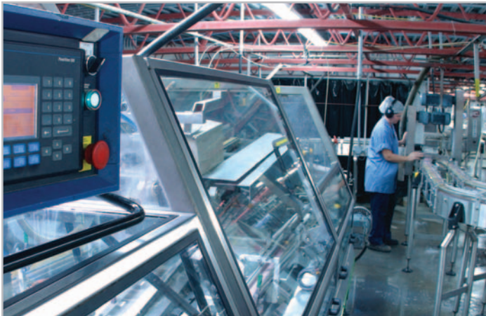
With today's advances in technology, companies can now fine tune almost every phase of production for maximum yield, quality and profit. At Leahy Orchards outside Montreal, Quebec, operator interface stations allow operators to quickly and easily monitor production status.
