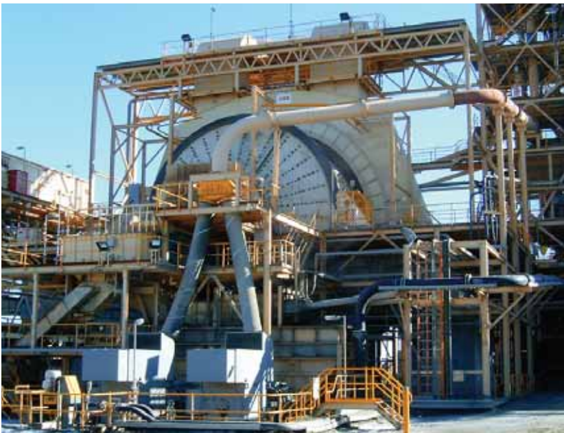
Integrated Condition Monitoring will provide a more accurate picture of the health of key machines, such as This SAG Mill.
